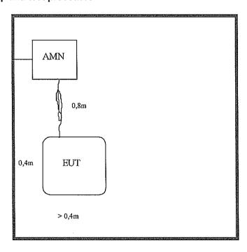
The mains terminal disturbance voltage was measured with the equipment under test (EUT) in a screened room. The EUT was connected to an artificial mains network (AMN), both were placed on a non-metallic table 0,8 m above a metallic, grounded floor. The EUT was placed 0,4 m from the reference ground plane (RGP) wall and 0,8 m from the AMN.
